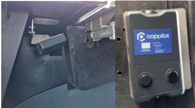
Figure 12: NES' sensors deployed inside waste containers.
