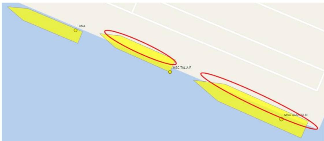
Figure 6.6: Detail of the mismatch between the vessel position and the GPS/AIS-reported position.
